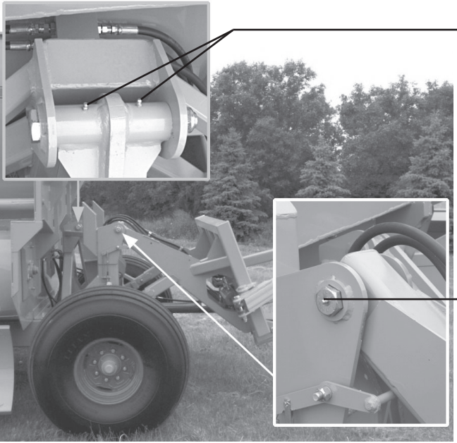
loader pivot lubrication points 1 & 2 of 4 (ref. 9)
