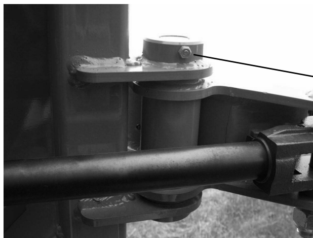
squeeze arm pivot lubrication points (one on each side of machine) (ref. 8)
