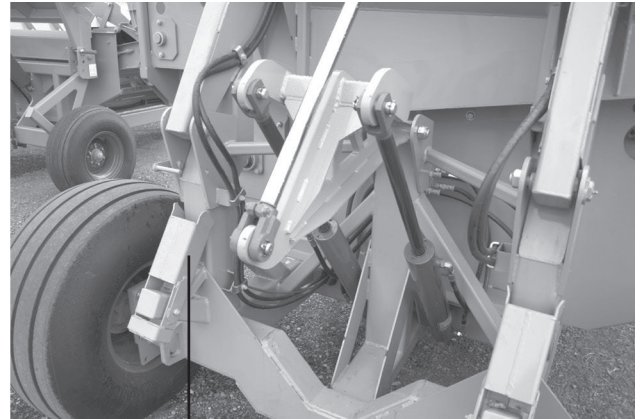
loader stops not in use
