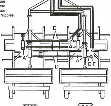
NOTE: Ball valves may be added to lift cylinders to operate drills individually.
